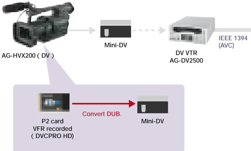
Record with a variable frame rate onto a P2 card, then dub it onto DV tape to achieve speed effects in your existing DV environment.
