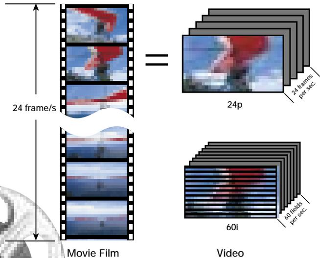
The film cameras used in making movies have a longer history than TV broadcasting cameras, and capture 24 frames per second onto silver halide film.
