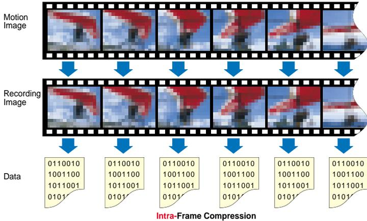
DVCPRO family: The data from each frame is compressed independently, so each frame can be reproduced singularly.
